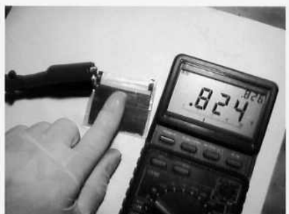
Two cells measures .824 vDC
