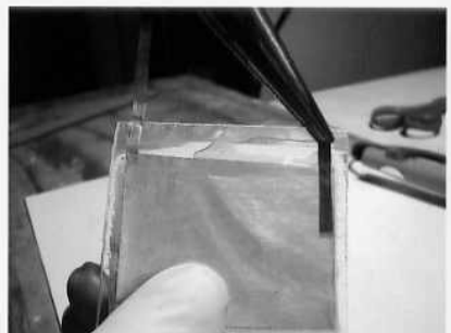
Bending back metal contacts
