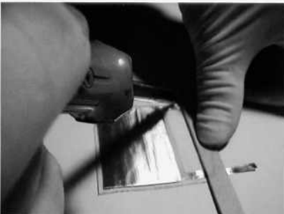
Sealing plastic with solder-iron
